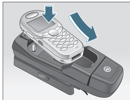
Fig. 13 Inserting the mobile phone into the phone adapter
